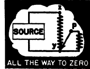
Action of a potentiometer.
